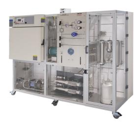
The 8500 Pressurized Foam Rheometer is designed specifically to measure the rheological properties of foamed systems under extended pressure and temperature conditions. The 8500 is a fully automated closed loop system that includes both hardware and software for the study of foam rheology over a wide range of foam qualities, shear rates and shear stresses.
