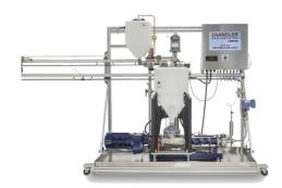
The 6700 Friction Flow Loop fully automated system includes hardware and software to measure the friction pressure of fluids. It determines the associated affects friction reducers have on fluids over a wide range of pressures and flow rate conditions and through different pipe diameters.
