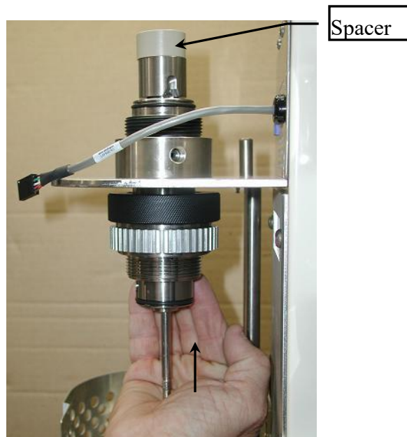
Figure 3-4 Bob Shaft Removal
