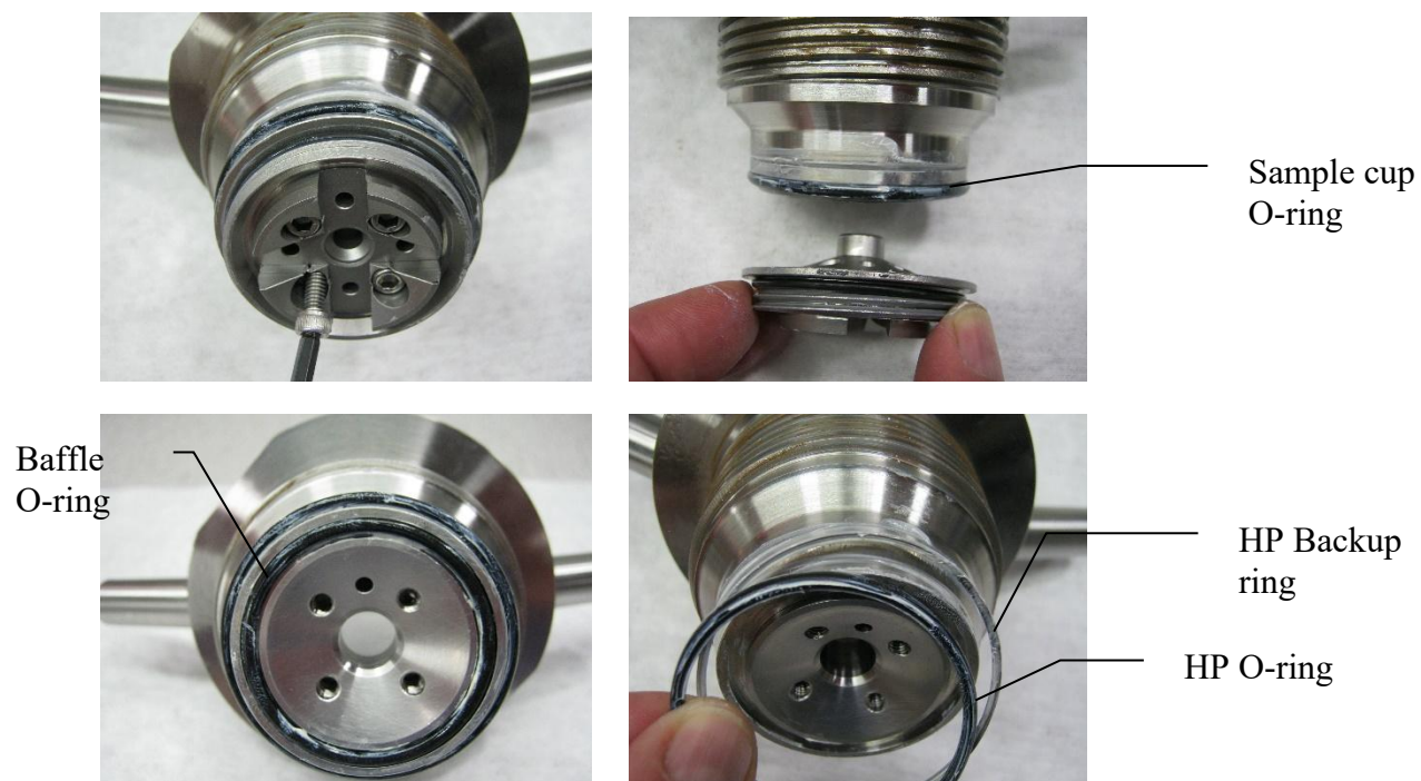
Figure 9 – Removal/Installation of Baffle and Seals
